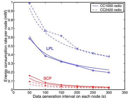
**Figure 9. Mean energy consumption rate (J/s or W) for each node as traffic rate varies (assuming optimal configuration and periodic traffic). The radios are the CC1000 (solid lines) and CC2420 (dashed).**
